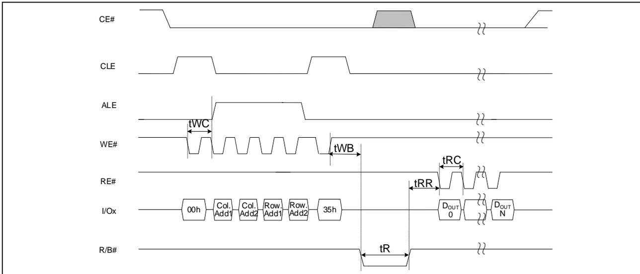
Figure 8-5: Copy-Back read sequential figures
