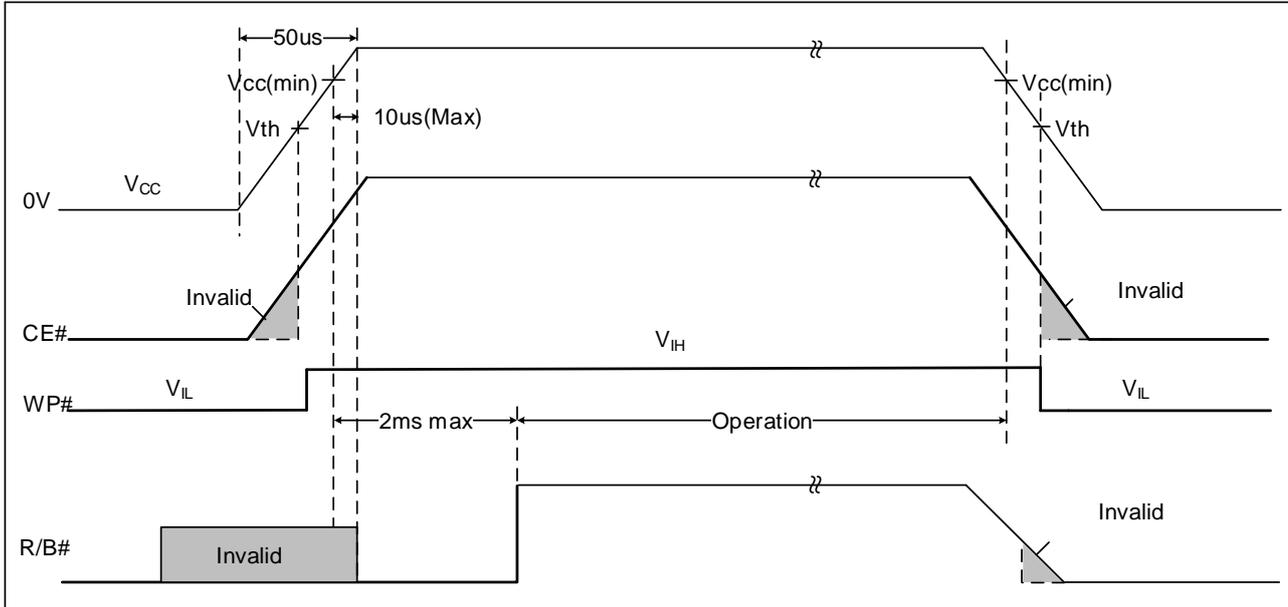
Figure 8-21: Data protection and Power on/off
