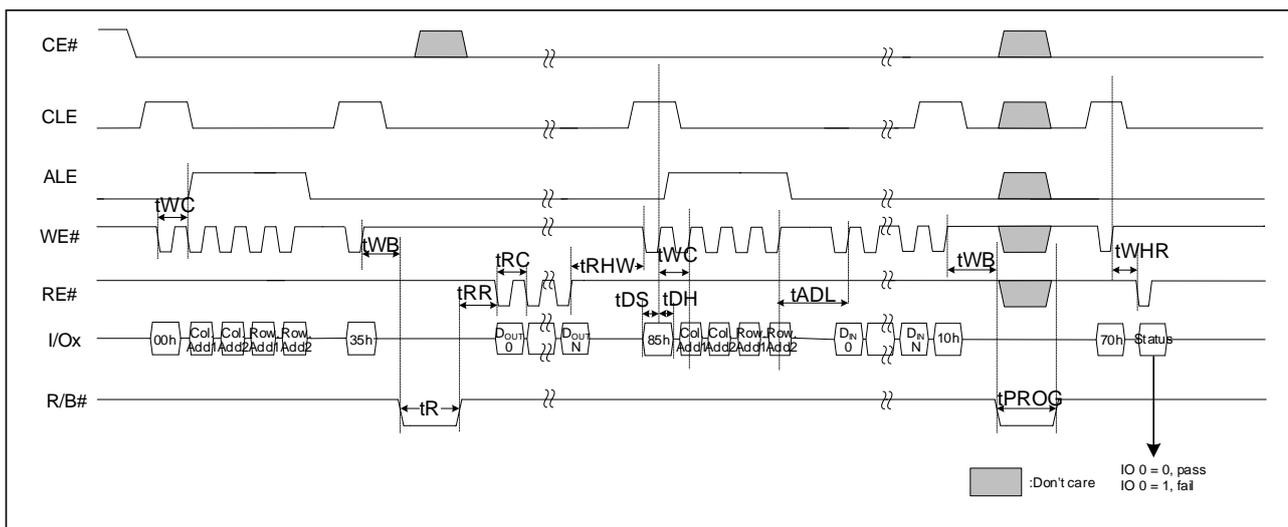
Figure 8-9: Copy-Back Program with Random Data Input figures
