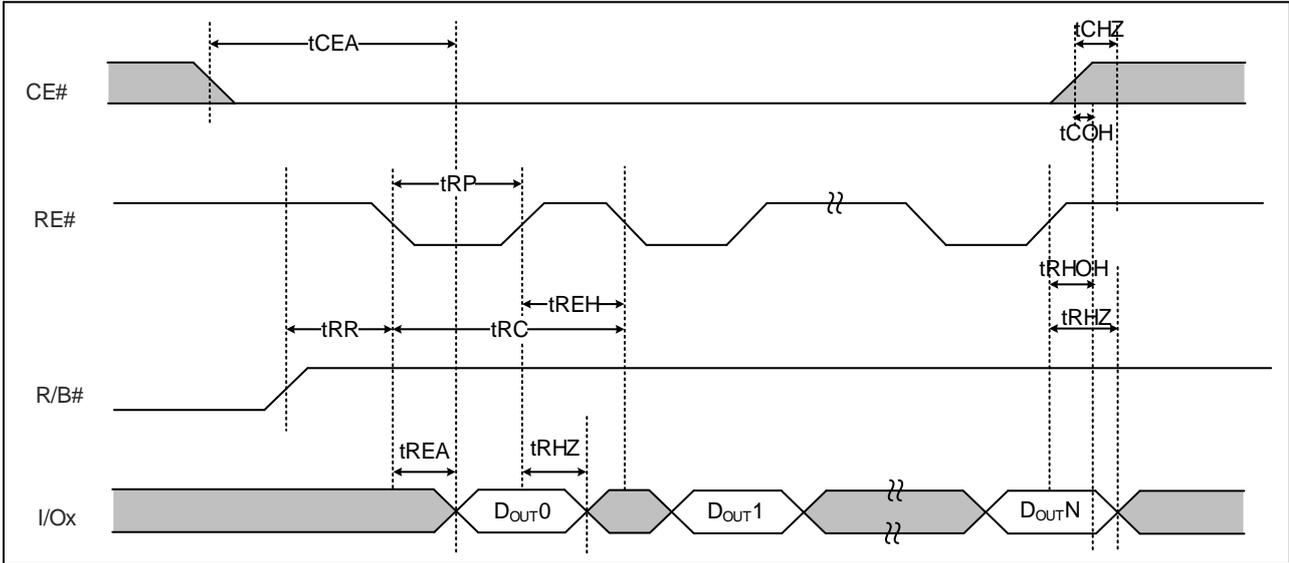
Figure 7-4\_a: Data Output Cycle figures
