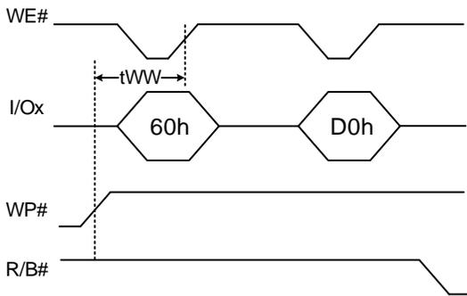
Figure 7-5\_c: Write Protect Disable with erase figures
