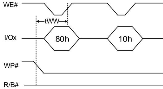
Figure 7-5\_b: Write Protect Enable with program figures
