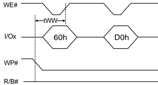
Figure 7-5\_d: Write Protect Enable with erase figures
