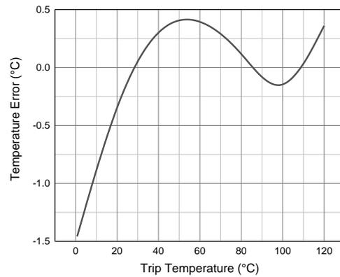
Figure 6. Temperature Error vs Trip Temperature
