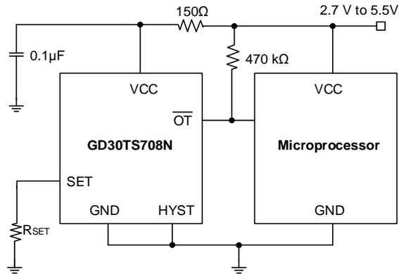
Figure 2. Typical Connections of the GD30TS708N
