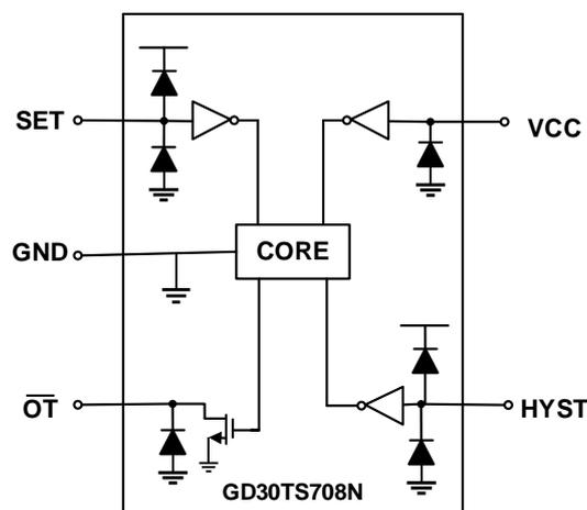
Figure 1. Equivalent Internal ESD Circuitry
